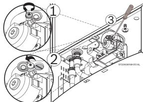
Fig. 55 Adjusting P1 CO<sub>2</sub> level
